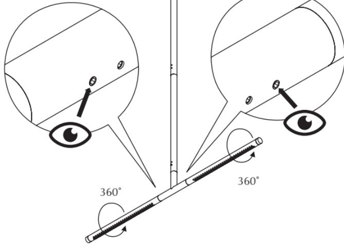
If screws are flushed with the surfaces, the arms can rotate freely.
