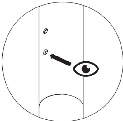
If screw is screwed into the tube, the arm is locked in the chosen direction.
