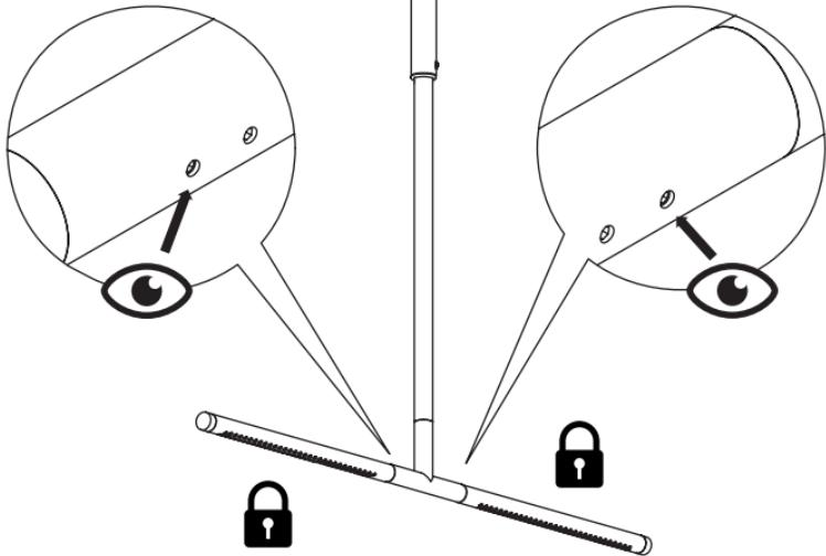
If screws are screwed into the tubes, the arms are locked in the chosen direction.
